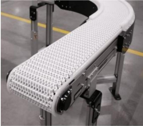
This simpler and safer conveyor belting is comprised of multiple polymer links that are releasably joined to one another to act like a fuse in the event of an overloading jam. Eminence manufactures innovative high performance and energy efficient modular plastic belt conveyor systems. Our low cost conveyor design combines direct drive motors and proprietary ultra-low friction plastic chain belting in a lightweight modular aluminium sectioned frame.
