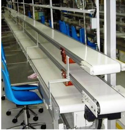
Belt Conveyor is a kind of machine that to transfer the material continuously. The belt works under the effect of frictional force. Eminence's Belt Conveyor is a kind of machine that to transfer the material continuously.
