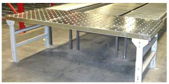
Ball transfer tables are ideal when you need manually to rotate or reposition products moving along conveyor belts. They can also be positioned where multiple lines meet, allowing you to move products more easily from one conveyor line to another.
